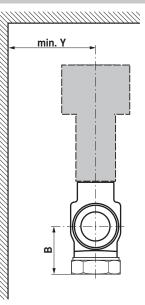
X/Y: Minimum distance with respect to the valve centre. The actuator dimensions can be found on the respective actuator data sheet.
