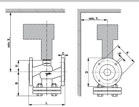
X/Y: Minimum distance with respect to the valve centre. The actuator dimensions can be found on the respective actuator data sheet.
