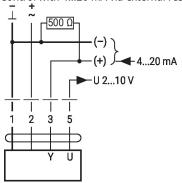
Override control with AC 24 V with Control remotely 0...100% with rotary switch
