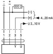
Override control with AC 24 V with Control remotely 0...100% with positioner SG.. rotary switch
